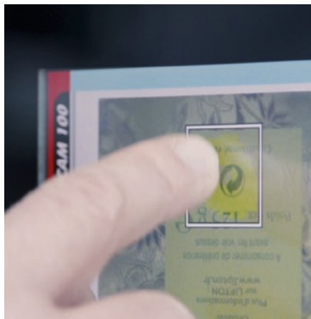
The control medium can be easily selected with a swiping touch on the 7" touch display.
