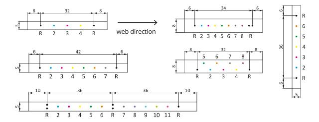
Examples of mark patterns (measurements in mm, not to scale), R = Reference mark
