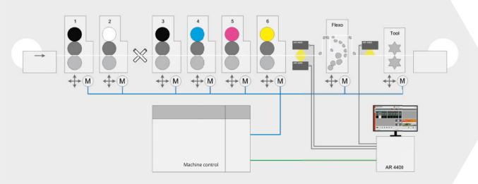
Example of a machine configuration for two-sided printing, an additional flexo unit and a cutting tool, all register controlled by the AR 4400.
