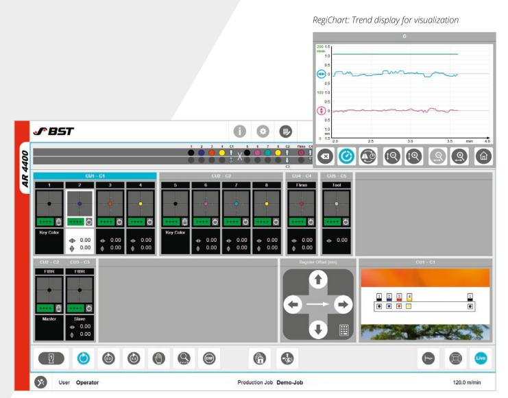
Touch screen for system operation and register display. The customized machine display makes system operation intuitive down to the smallest detail.
